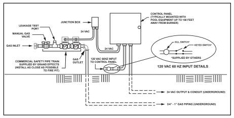
Figure 3. Commercial Installation
