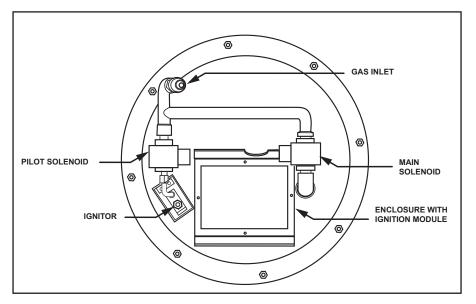
Figure 9. Bottom-side of Burner Assembly
